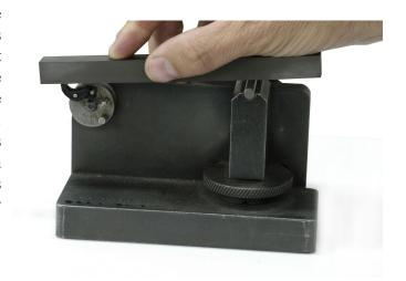
Stone the hammer sear hooks with the fine India stone only. This will smooth up the 90 degree hooks to a mirror finish. With the medium Arkansas stone, take the height of the hooks down to 0.020". This is the height of the feeler gauge (shim) that comes with the jig.
