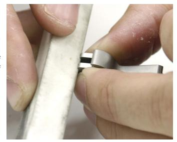
Bend the sear spring to remove some of its tension. We always try to keep the disconnector (center) leaf and the sear (left) leaf the same height at the top, no matter where they have to be. You need to always make certain the disconnector snaps up positively, and the sear moves freely to block the hammer from falling. This will take a bit of trial and error to find out what works best with your particular set up.
