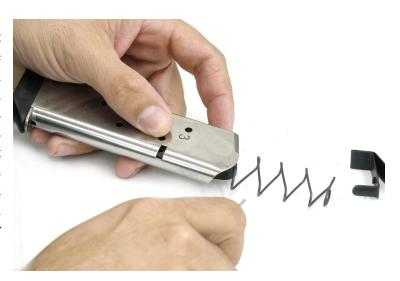
Clean the spring, follower, and inside of the magazine tube thoroughly with solvent and reassemble in reverse order. Install the spring first and make sure the raised portion of the spring faces toward the front of the magazine. Then depress the spring into the tube with your blunt object so that it can be captured with the punch the third hole down.
