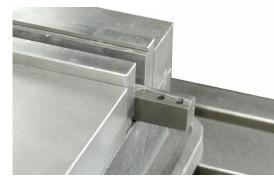
3. Center the machine spindle over outermost hole in the jig. Depending on how close you like to work, this can be indicated in precisely, or merely run a 5/32 (.1565) drill or reamer through to center it up. We highly recommend you use the most accurate method you have, as this hole location is critical to a good job.
