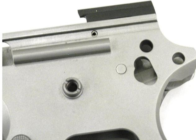
File a small flat on the front of the ejector so that any sharp corner is removed. Make this flat exactly perpendicular to the frame top. If a sharp corner was left here, it could mark the brass, or get pushed over where it could possibly contact the moving slide. I suppose it is not impossible to speculate that such a sharp corner could fire a loaded round. Stranger events have occurred.
