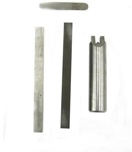
Complete instructions are included with our jig, but basically you stone the top of the sear with the medium Arkansas stone until the surface is flat clear across. Do not take off any more than necessary, and make sure the included shim is in place. Once the angle is set, rub it firmly with the fine India stone to get a mirror surface. Note the left index finger is holding the sear securely against the adjustable screw stop.
