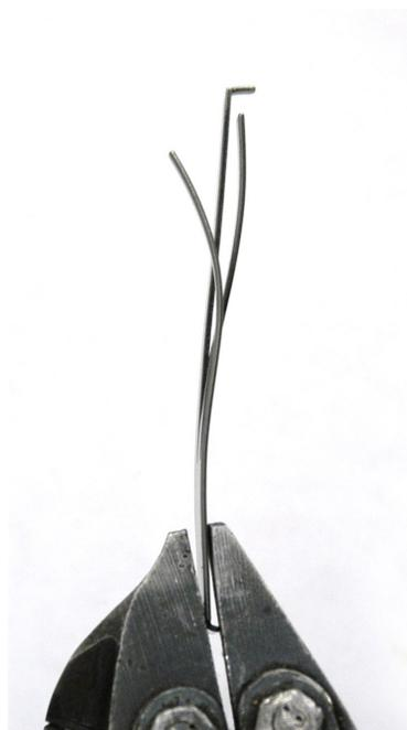
Reassemble the pistol's basic components and try out the new trigger. If it is still too heavy, try to bend the sear spring a bit straighter, then reassemble and try again. If the trigger has too much creep, stone a bit more 45 degree clearance on the sear. Pull weight should be set by a trigger-pull scale, or lifting a trigger-pull set of weights. We use both in the shop, but I prefer to use the weights.
