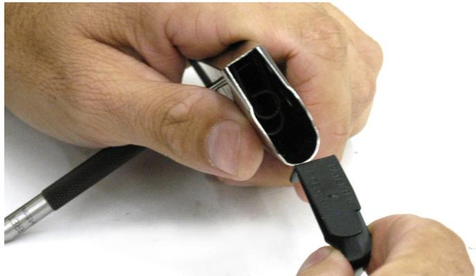
Once the follower is removed, turn the magazine upside down, so the spring doesn't fly away, and pull the pin out to release the spring.
