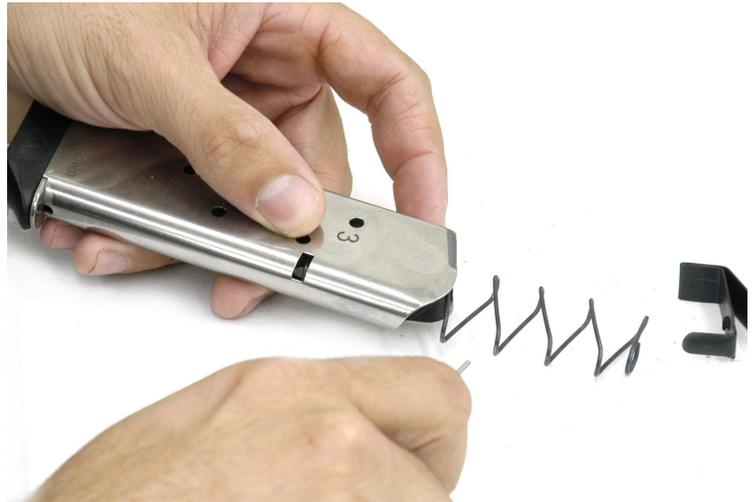
Clean the spring, follower, and inside of the magazine tube thoroughly with solvent and reassemble in reverse order. Install the spring first and make sure the raised portion of the spring faces toward the front of the magazine. Then depress the spring into the tube with your blunt object so that it can be captured with the punch the third hole down.
