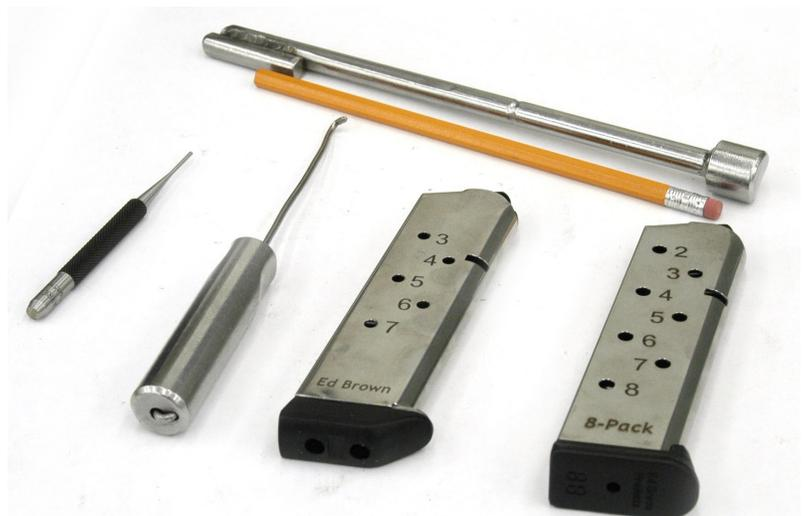
To disassemble the magazine, depress the follower with the blunt object and press it down to a point where it can be seen below the third hole from the top. Then let it raise back up until you can capture the spring just below it. Insert the punch completely through the magazine and release the pressure on the follower. Now the spring is captured and the follower can be removed.
