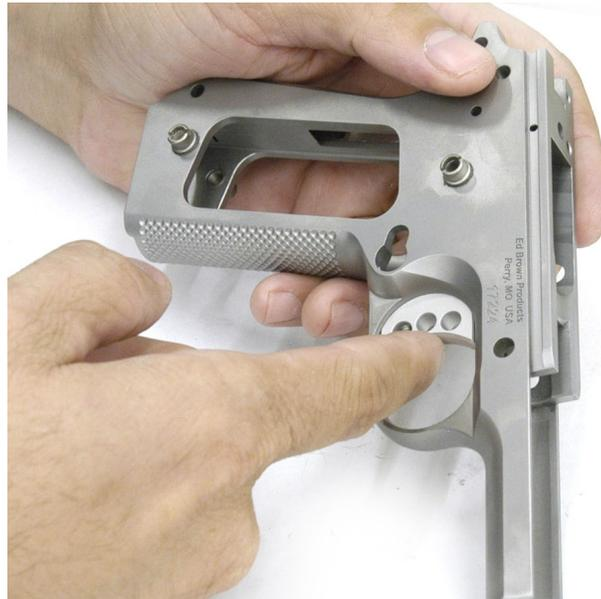
Continue working until the trigger will move smoothly in and out without any binding. A good check for trigger operation is to hold the frame muzzle down and lift the trigger and let go. It should drop fully forward under its own weight without binding.
