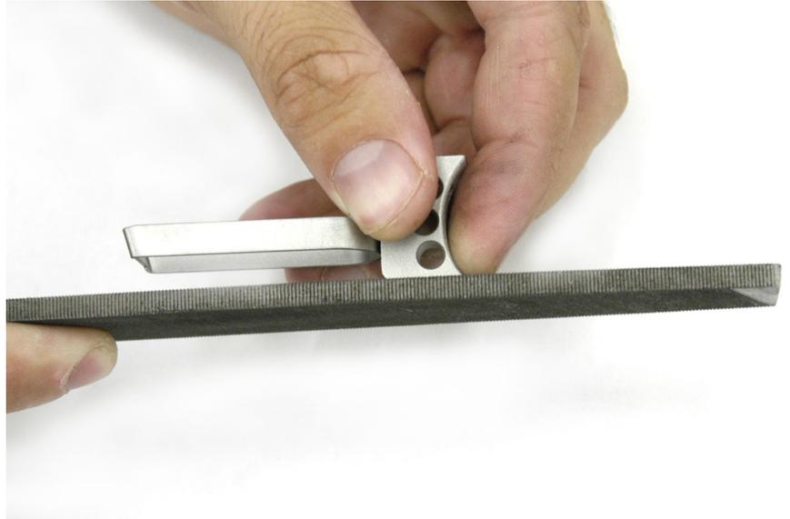
You will probably determine that the top and bottom surfaces will need a little metal removed. Hold the trigger firmly, as shown in the photo, and slowly file some material away. A 3/4" wide file works great for this. Go slowly and keep the surface flat and even. Remove about the same amount from the bottom and retry the fit.
