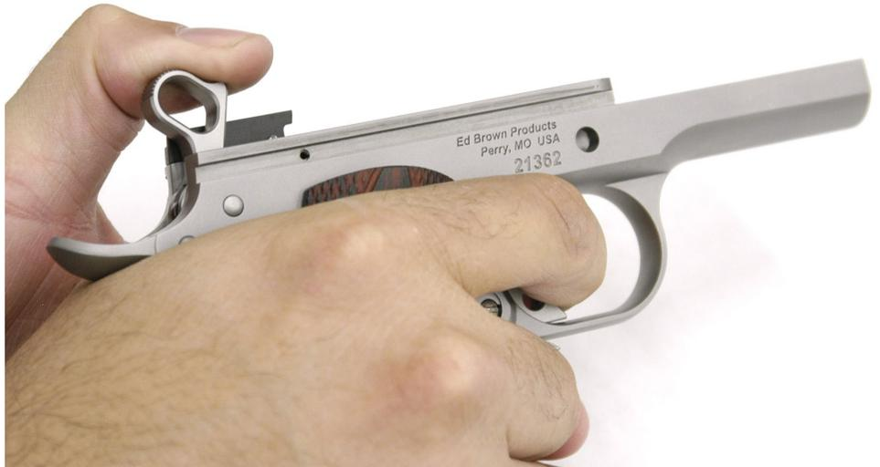
If the hammer will not go all the way down, or if you can feel the hammer rub the disconnecter, the over-travel screw is too tight. Back it off. If nothing can be felt after the release, you can tighten the over-travel screw about 1/4 turn and try again. I usually tighten the screw until a slight rub is felt, and then loosen the screw about 1/8 to 1/4 turn.
